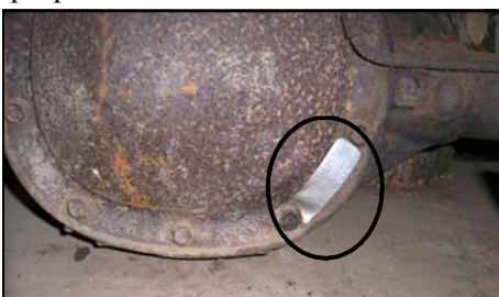
Tag identifying axle as Positraction
