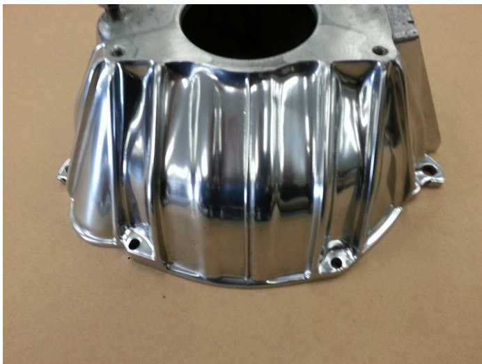
Chris Wheaton's latest project? Getting some headers coated in three different colors! Below is a polished Bell Housing ceramic clear coated. Could be a good process for bumpers!
