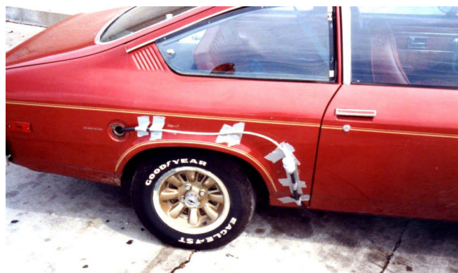
Functional repair to bypass a bad in tank fuel pump! Dave Elliot had to do this to get his CV home from the 1990 Green Bay Roundup!
