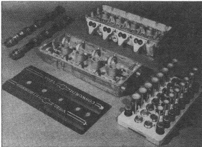
Twincam valve train: separate aluminum cam carrier (center) and head (upper right) replace one-piece cast iron head of standard Vega.
