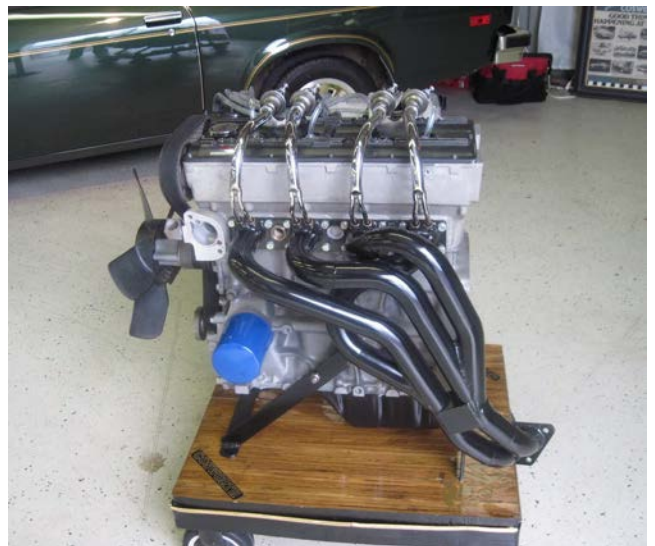
Jack pulls out another trick out of his hat for Roundup 32. This display only Cosworth Vega 2.0 liter engine is mounted on a wooden stand with wheels for easy moving. The engine turned out to be a big hit with Building T visitors.
