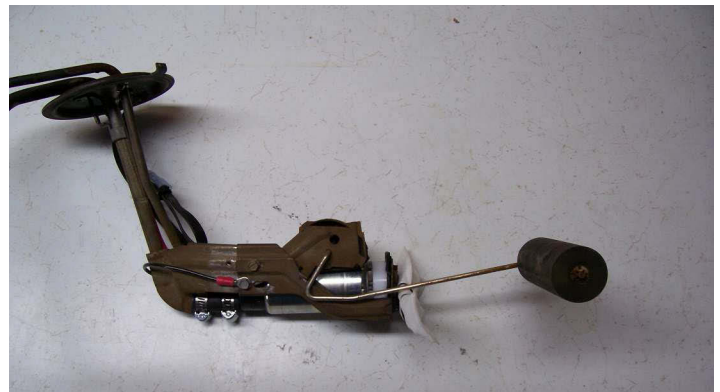
Assembled fuel pump and sender unit with the float lever in the empty position.
