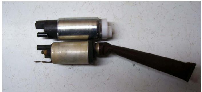
The low pressure CV pump next to the Fiero pump. As you can see, the Fiero pump is about 3/4" longer than the CV unit.
