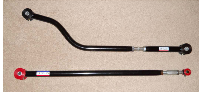
Spohn Performance adjustable Panhard arms for H-body cars. The arm for '75 model year cars is on top, the '76 on the bottom.
