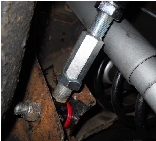
Adjuster threads and sleeve of the Spohn Panhard arm. The picture angle makes it look like shock clearance is tight, but it is really not.
