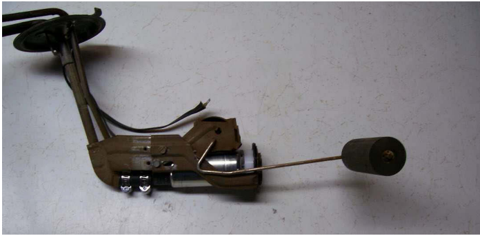
Pump assembled mounted on the bracket. Note that two new holes must be drilled for the screws.
