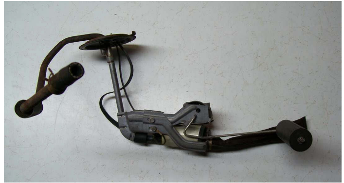
Stock configuration of the low pressure pump and the fuel gauge sender as removed from the tank.
