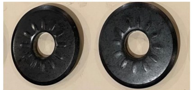
Front Lower Control Arm Bushing End Caps - Ferrules
