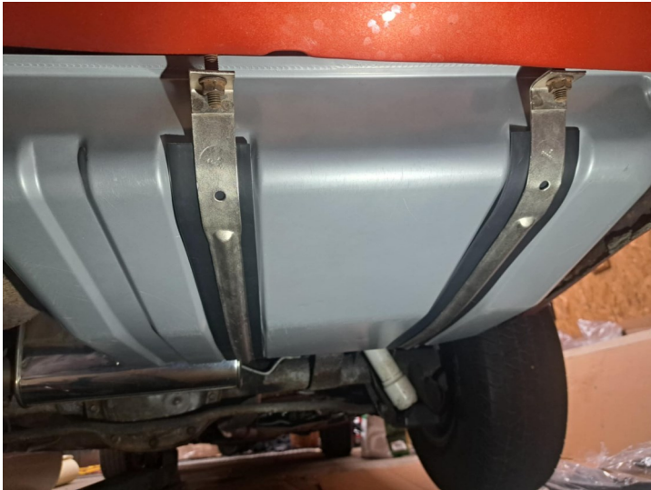
Test Fit of Second Sample Tanks with Clyde Biagi Gas Tank Strap Kit.
