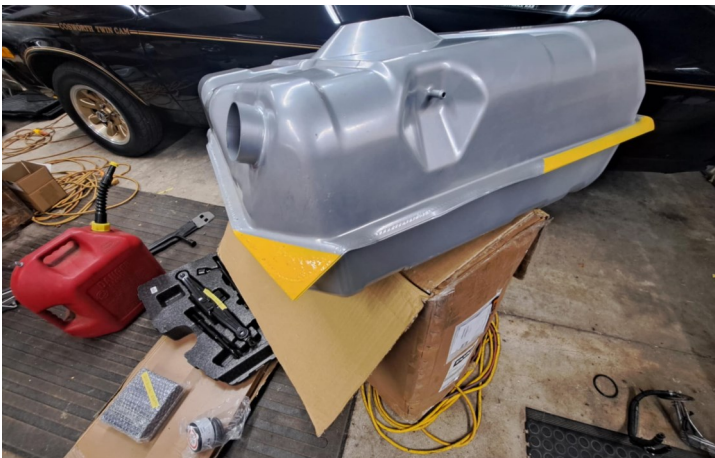
Test Fit of Original Sample. Identified corner and edges not bent down enough.. This is why you test fit! (Been Corrected!)
