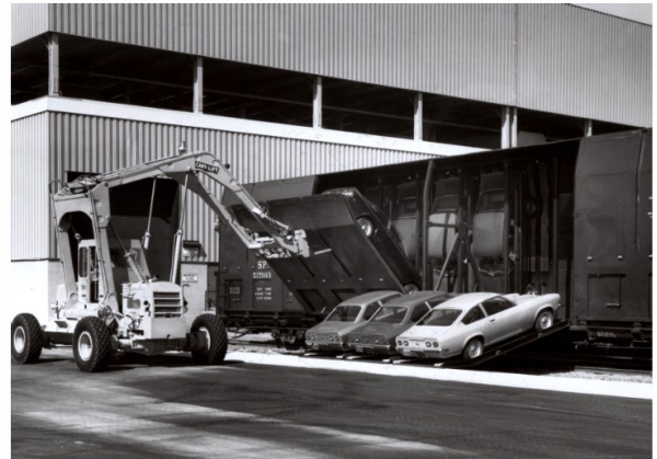
The Vert-A-Pac rail loading area, where Vegas were shipped, 30 to each special rail car, nose-down and fully protected from the elements and vandalism. Four cast iron sockets were inserted in reinforced holes in the underbody, then the cars were driven onto the lowered rail car door; when the rail car door was raised, the cars rolled a few inches forward and the sockets engaged four steel hooks on the rail car door.
