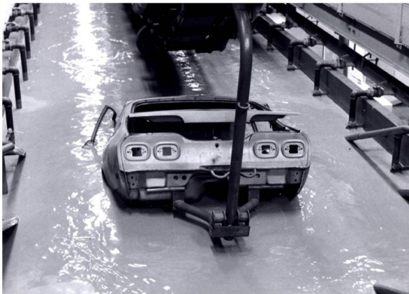
Vega entering the 65,000-gallon "ELPO" dip prime tank after numerous cleaning and phosphating stages; the body is charged negatively at high voltage, and the primer tank is positively charged to ensure full and evenly-distributed film build throughout the body structure. Clamps were added to the conveyor hangers later to avoid bodies "floating" off the hangers and sinking in the tank.
