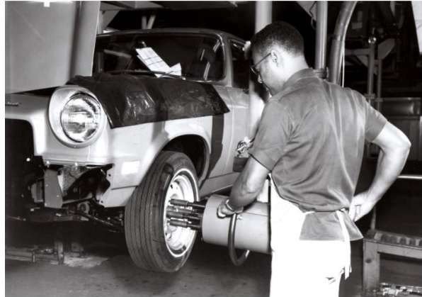
Tire and wheel installation, using a multiple nutrunner. Tires were mounted and balanced in an automated system across the aisle at 550 assemblies per hour and delivered by overhead roller conveyors to the assembler in the roller chute at lower right; the fifth (spare) tire was diverted to another conveyor chute much further down the line for installation with the car at floor level. Note the machine-readable traveling inspection ticket under the windshield wiper, and the undercoating in the wheel well (sprayed in a booth in the background).
