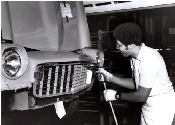
Grille installation - note plastic spacers to center it; the plastic nuts that accepted the grille screws were white so the assembler could see them clearly through the screw holes in the grille. Note the half-size broadcast sheet taped to the hood; teletype printers of the time couldn't print full 8.5"x11" sheets at 102 units per hour, so two separate half-length sheets were created. The one on the hood is the "Body" broadcast, and the one below the grille is the "Chassis" broadcast; each carried unique and separate information for those assembly areas.
