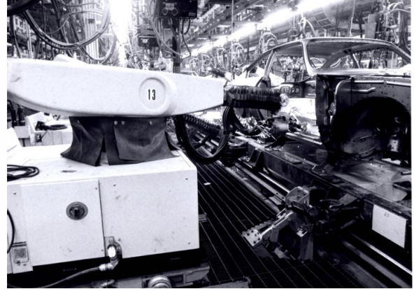
Unimate robot in action – the large device at the lower right is a hydraulically-operated toggle that locks the body build truck in position before the robot begins its welding cycle. The robots are mounted on tracks so they can be easily pulled back from the line for access for preventive maintenance from the aisle.
