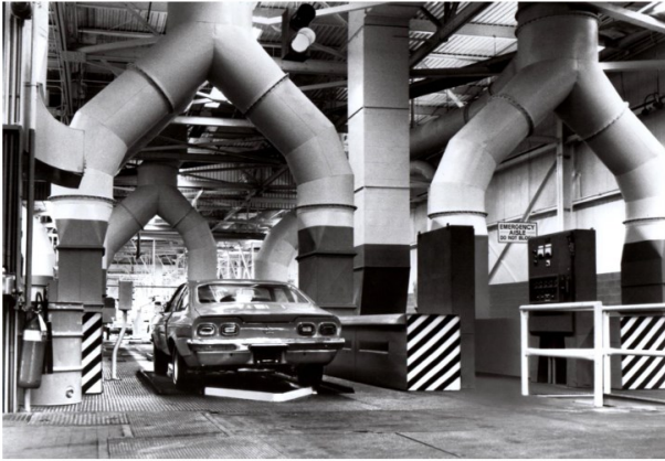
One lane (of four lanes) of the final functional test section as the Vega came off the line. The first test was a road simulator with four independent hydraulic cylinders that shook the car with the engine off to spot any squeaks or rattles, the second was a brake tester that measured braking force at each wheel as the driver drove in and stomped on the brakes, and the third was a dynamic roll-test where the car was driven on rollers at road speed and then had toe-in set with the front wheels turning. Massive ductwork draws exhaust fumes out of the area.
