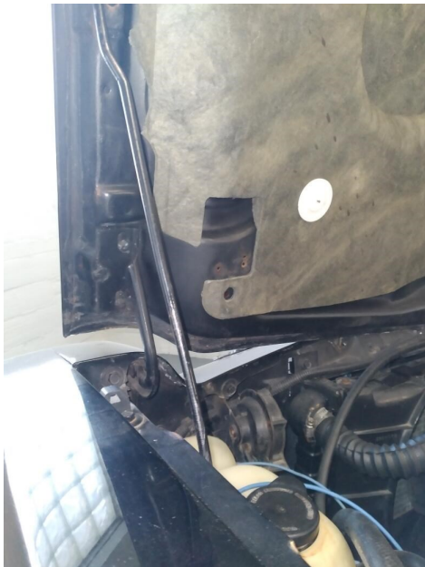
Starting Point w/ Lt. Fix Rem'l Inner Hood Pnl. @ Washer Bot
