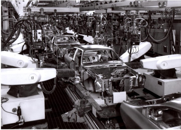
The "Unimate Line", the first fully-robotic automated body welding line in the industry; 26 Unimate hydraulic robots in 11 stations completed all body structural welding following body framing. Each body build truck weighed 14,000 pounds, and the conveyor drive system shuttled the entire line in unison from station to station every 30 seconds (120 units per hour).
