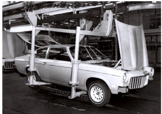
Nearly-completed Vega preparing to transfer from the overhead conveyor to the moving "Flat-Top" floor conveyor plates on the Final Assembly Line; the rollers under the car center it for proper positioning on the conveyor.
