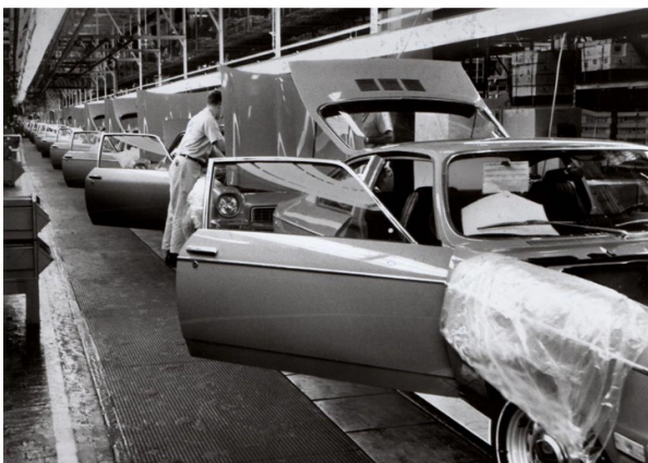
Nearing the end of the Final Line - in a major departure from traditional practice, Vega seats were assembled across the aisle and were installed last to provide better assembly access to the interior of the car all the way through the assembly process. Front seat installation was simplified by having studs on the tracks that went through holes in the floor, and the nuts were secured from the center pit area between the conveyor tracks.
