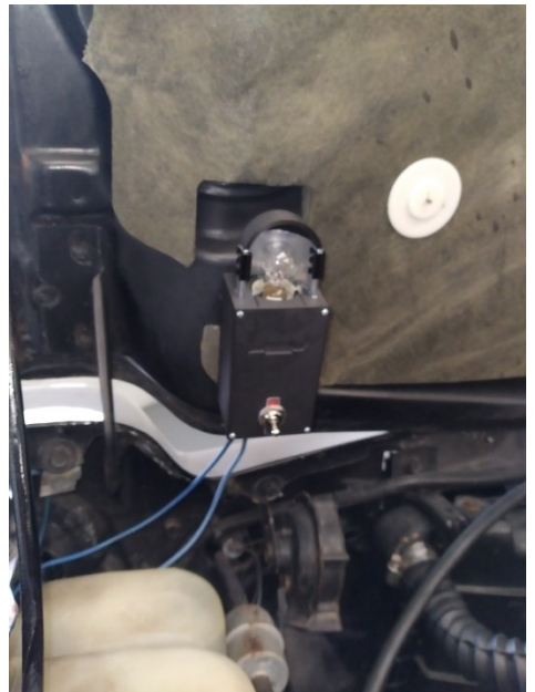
Finish Product Mtd. & Wired w/ On-Off Sw. (Dorman #85982 Switch)
