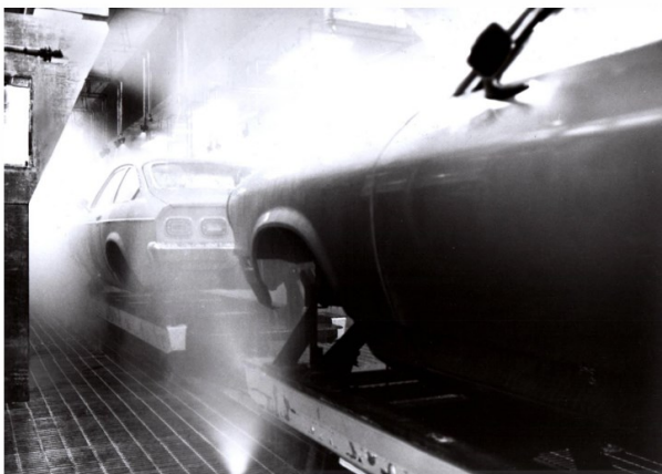
Four-minute deluge full-body water-test in the Trim Shop; the water contained a special dye that showed up under ultraviolet light in order to trace the source of any leaks.
