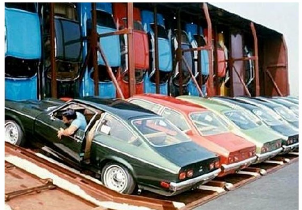
Vert-A-Pac was only used for Westbound shipments, as most railroad underpasses on the East Coast were too low to clear the very tall Vert-A-Pac rail cars; Eastbound rail shipments used conventional tri-level rail cars. Vert-A-Pac was a joint venture between GM and the Southern Pacific Railroad; the railroad supplied the basic "chassis" of the rail car, and GM paid for all the structure and mechanisms from there up.
