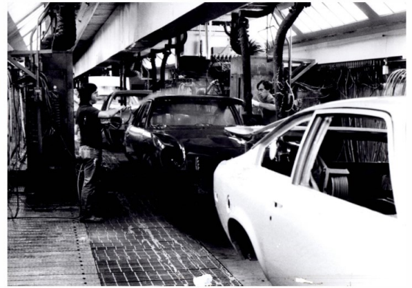
Main downdraft exterior color spray booth; the interior has already been painted trim color and has been masked off (note masking paper on the dash of the dark car in the center of the photo). Note quick-color-change hoses and manifolds on the wall behind the sprayers. Ideally, colors were "batched" for two or three units in a row of the same color, as each color change sent about $2.00 worth of lacquer and solvent down the drain to flush the lines to the spray guns.
