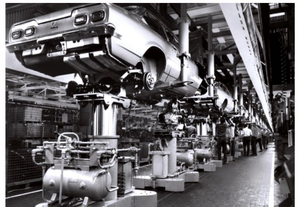
View of the main portion of the Towveyor Line; the unit in the foreground shows the rear axle nearly in position (note rear coil spring in position on the base of the Towveyor for the assembler). Fuel tank was installed earlier, exhaust system was installed further down the overhead line.
