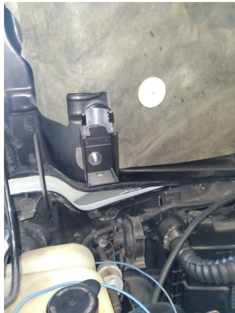
Redesigned Lt. Fix. Mount'g Utiliz'g Hd. Pad Push Pin Loc. (Held-in-Place 1/4" `L' Bolt)
