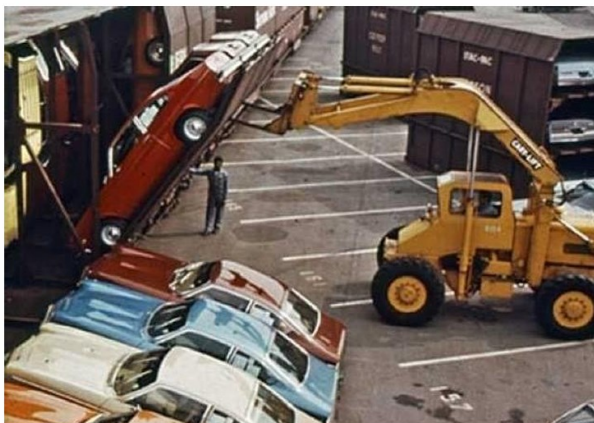
All Vega fluid containers (fuel tank, carburetor, battery, washer fluid, engine crankcase, etc.) were designed so the vent locations were above their fluid levels whether the car was level or standing vertically on its nose. Note the traditional tri-level Stac-Pac rail cars on the right which could only hold up to 15 cars vs 30 cars with Vert-A-Pac.
